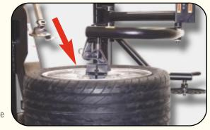
operator in seating the rim clamp jaws between the tire and the outside rim on difficult to depress stiff sidewalls.
