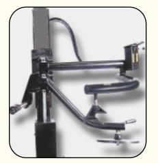
Wheel Centering Depressor – This slide-on depressor provides downward pressure on the rim when clamping low profile tire and rims, assists
