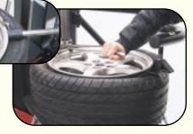
Power push up disk lifts tire up on the rim so the operator can more easily demount the tire.
