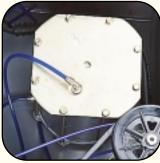
Rust-Proof Drive Cylinder • Critical bead breaking cylinder is lined with rust-proof polyfiber liner for years of rust-free operation. • Non-lined cylinders will pit, causing
